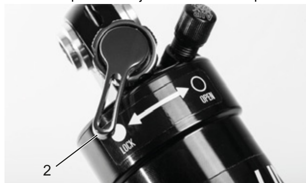
Figure 66: Suntour compression adjuster closed (2)
