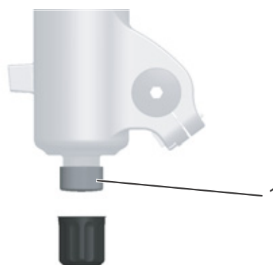
Figure 54: FOX rebound adjuster (1) on the fork
