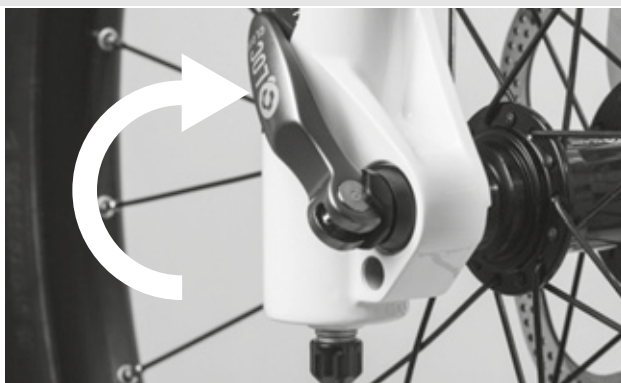
Figure 35: Closing the quick release
