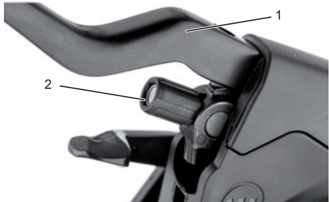
Figure 76: Brake lever (1) of the hydraulically operated rim brake with setting bolt (2)
