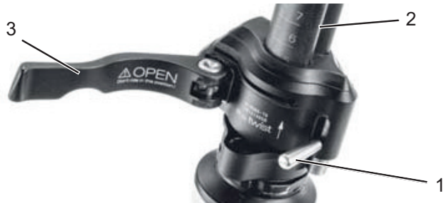
Figure 61: Opened clamping lever on the stem quick release (3) on the stem (2), version I, with locking lever on the stem (1)
