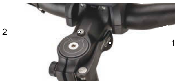
Figure 139: Stem, version II with clamping lever on the stem quick release (1) and unlocking knob (2)
