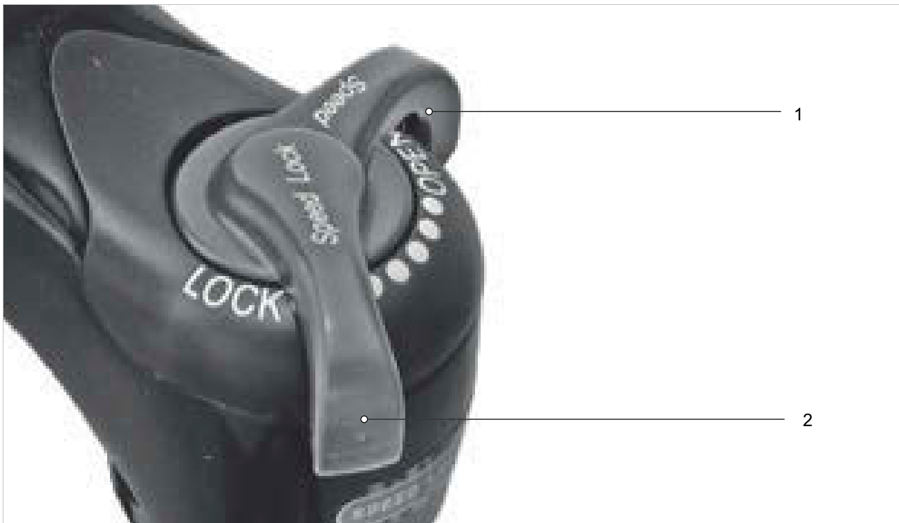
Figure 135: SR SUNTOUR compression adjuster in open (1) and closed (2) position
