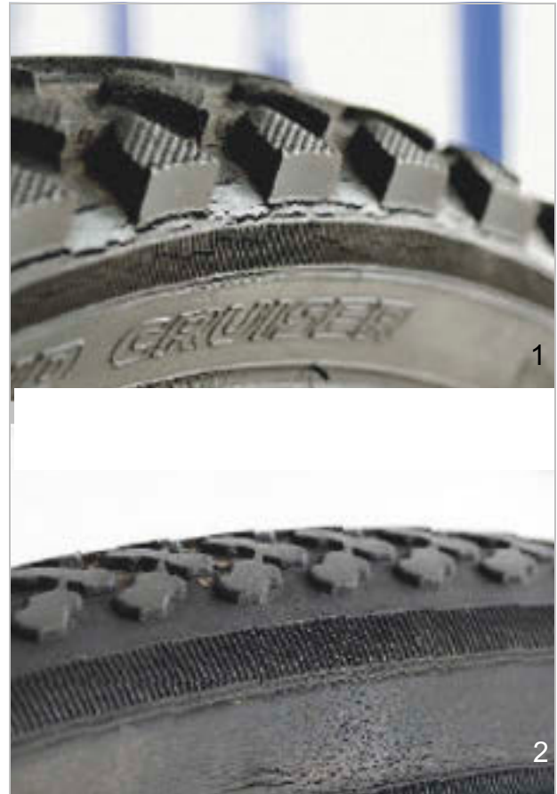
Figure 152: Examples of fatigue cracks (1) and ageing cracks (2)
