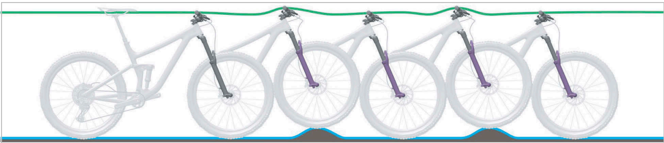
Figure 12: Optimum suspension fork ride performance
