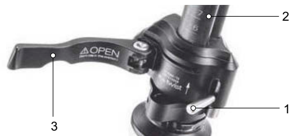
Figure 138: Opened clamping lever on the stem quick release (3) on the stem (2), version I, with locking lever on the stem (1)
