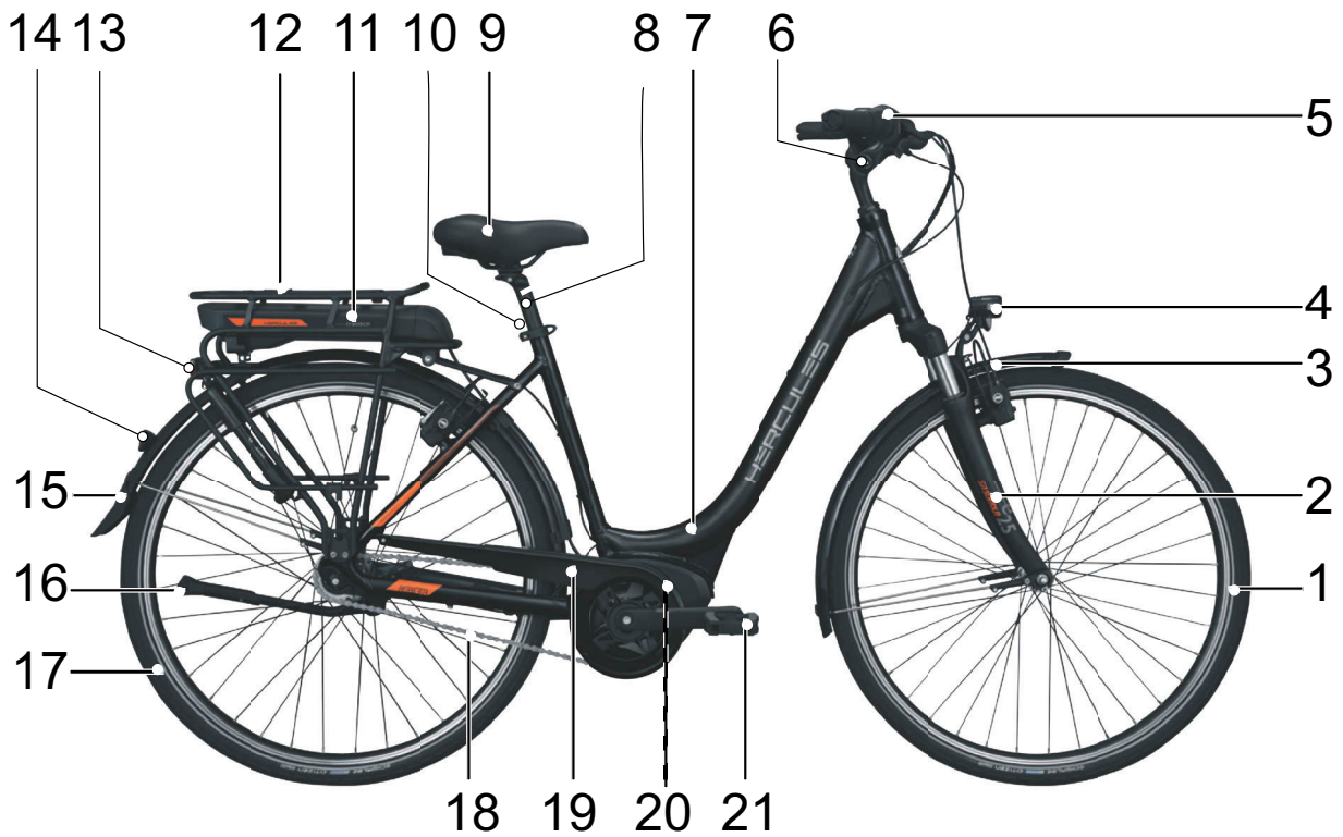
Figure 3: Pedelec viewed from right, HERCULES Futura Sport I 9 used as example
