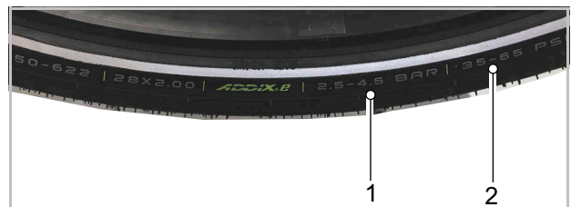
Figure 150: Tyre pressure specification in bar (1) and psi (2)
