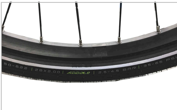
Figure 20: Example: Information on tyres
