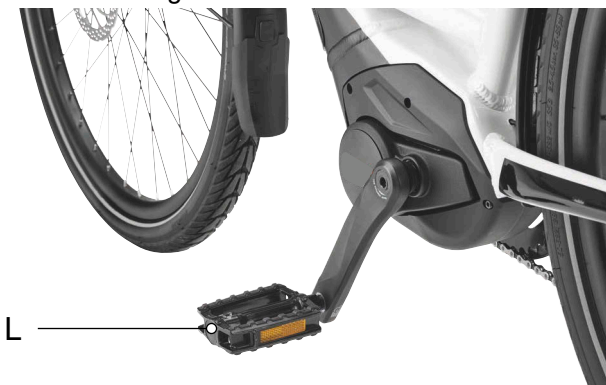
Figure 53: L pedal in the left-hand crank arm
