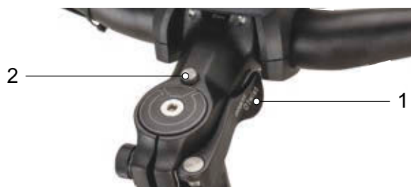
Figure 51: Stem, version II with clamping lever on the stem quick release (1) and unlocking knob (2)
