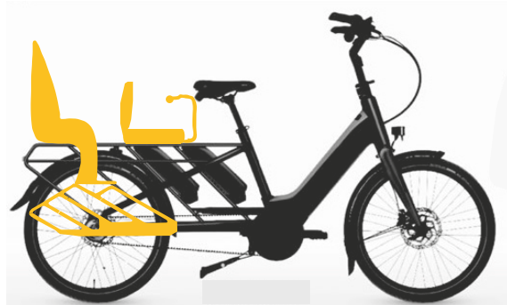
Figure 97: A child seat at the rear and a saddle seat with sideblades in front, suitable for one young child (1–6 years old, 9–22 kg) and an older child (6–10 years old, 18–38 kg)
