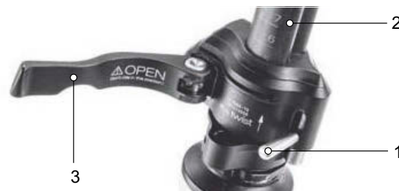
Figure 201: Opened clamping lever on the stem quick release (3) on the stem (2), version I, with locking lever on the stem (1)
