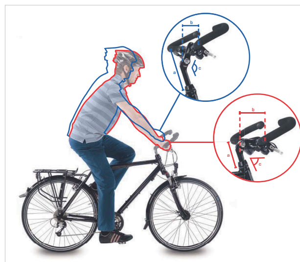
Figure 136: City bike (blue) and trekking bike position (red) by changing the angle
