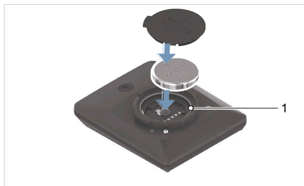
Figure 162: Inserting the battery with the seal rubber (1) aligned correctly
