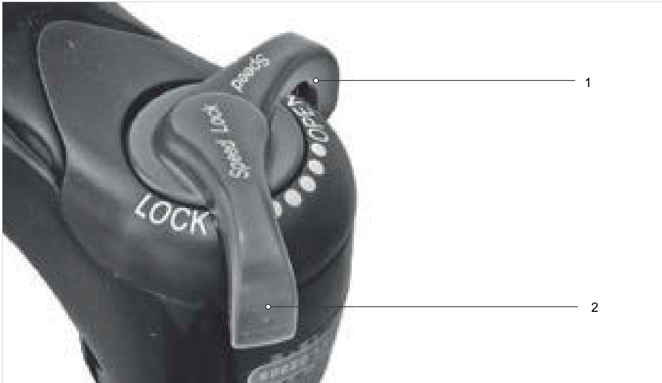
Figure 198: SR SUNTOUR compression adjuster in open (1) and closed (2) position
