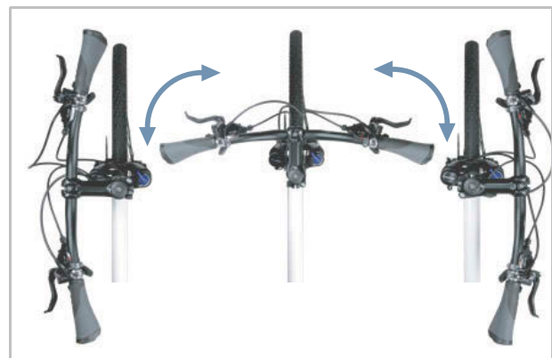
Figure 10: Twist function, using BY.SCHULZ as an example
