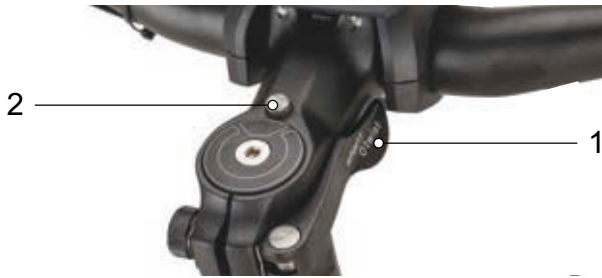
Figure 202: Stem, version II with clamping lever on the stem quick release (1) and unlocking knob (2)
