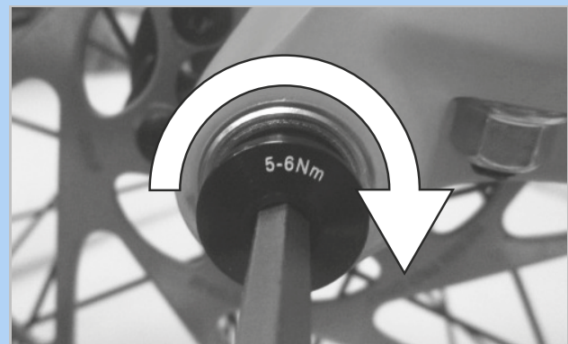
Figure 101: Tightening the securing screw
