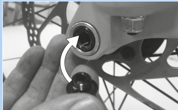
Figure 63: Inserting the securing screw
