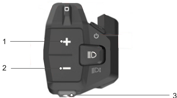
Figure 150: Position of plus button (1), minus button (2) and push assist button (3)
