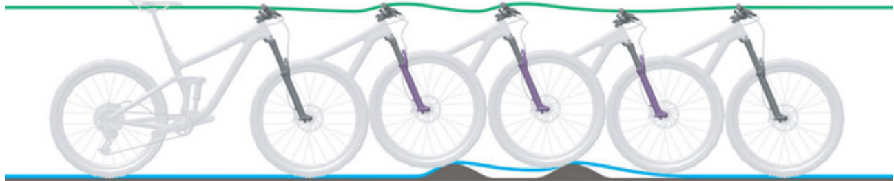
Figure 217: Suspension fork rebounding too slowly
