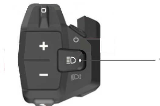
Figure 149: Position of riding light button
