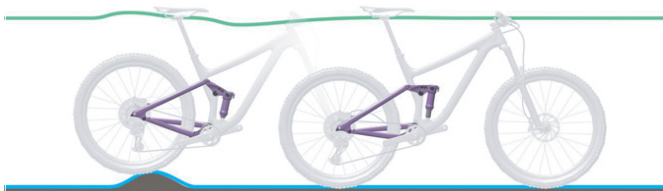
Figure 125: Optimum rear frame damper ride performance over bumps
