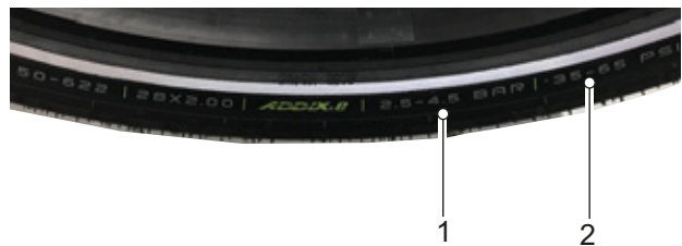
Figure 164: Tyre pressure in bar (1) and psi (2)
