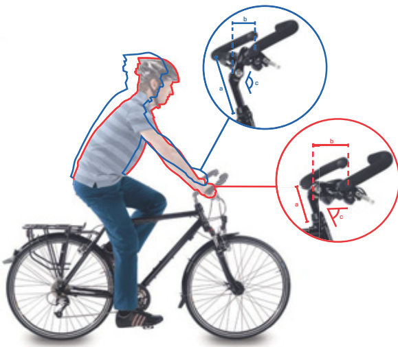
Figure 110: City bike (blue) and trekking bike position (red) by changing the angle
