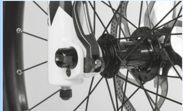
Figure 195: Adjusting the quick release clamping force
