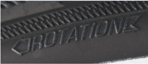
Figure 59: Rotation direction arrow
