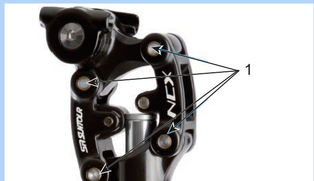
Figure 197: SR SUNTOUR suspension seat post lubrication points
