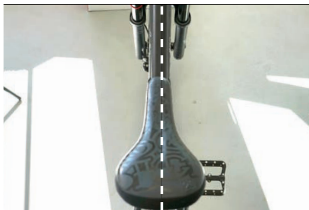
Figure 95: Positioning the saddle in direction of travel
