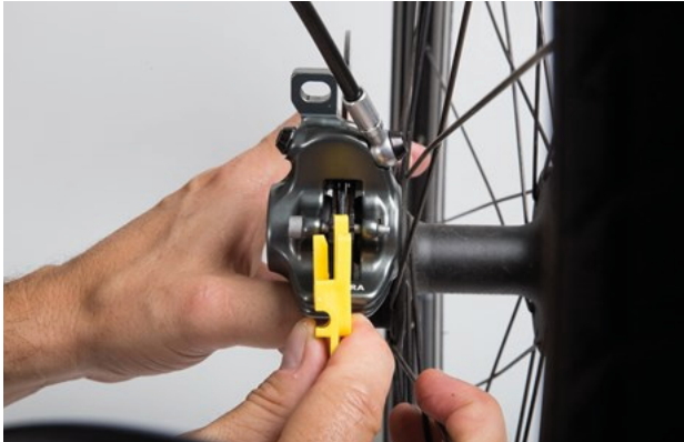
Figure 167: Checking the brake lining when fitted with the help of the transport safety wear gauge
