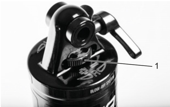
Figure 228: SR SUNTOUR rebound adjuster wheel (1) on the rear frame damper
