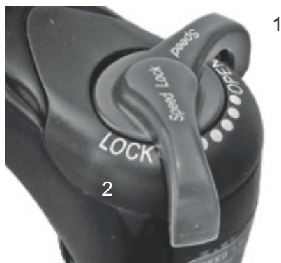
Figure 80: Suntour compression adjuster with the OPEN (1) and LOCK (2) positions
