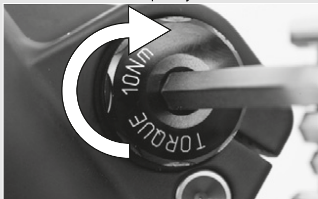
Figure 30: Tightening the inserted axle
