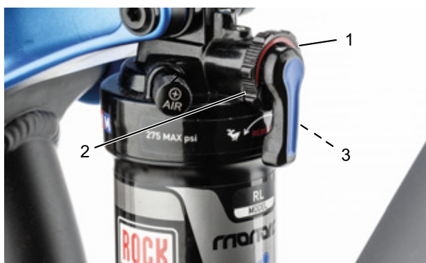
Figure 83: Setting the rebound damper strength on the rear frame damper setting wheel (1)
