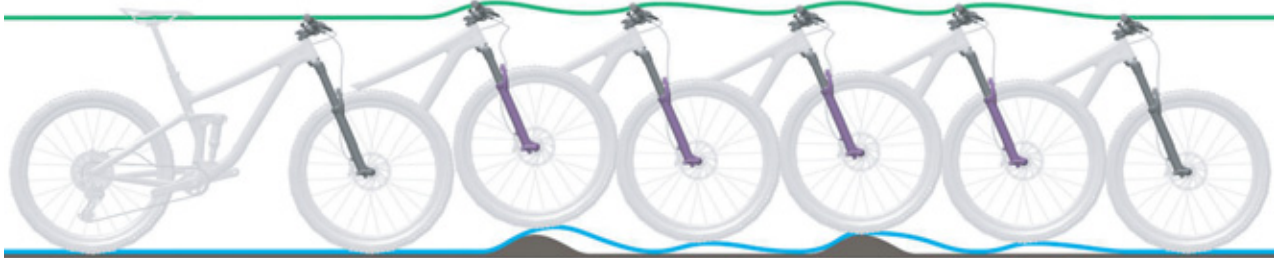
Figure 211: Suspension fork rebounding too quickly
