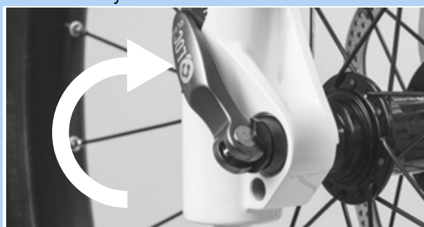
Figure 84: Closing the quick release
