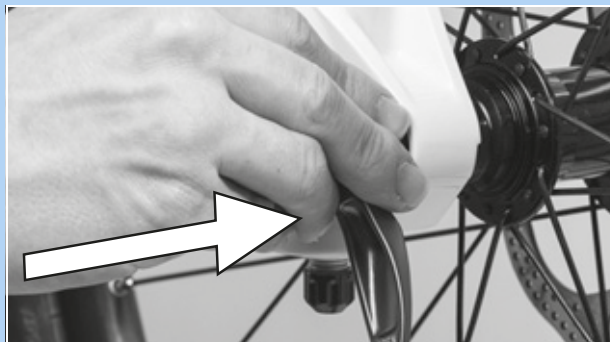
Figure 82: Inserting the quick release in the direction of the arrow
