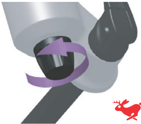
Figure 214: Turning the rebound screw damper towards hare symbol
