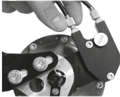
Figure 196: The tension adjuster on ROHLOFF hub versions with external switch control is located on the cable box positioned on the left-hand side
