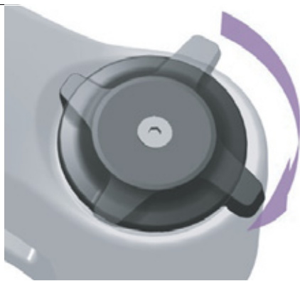
Figure 216: Changing compression adjuster to a harder setting
