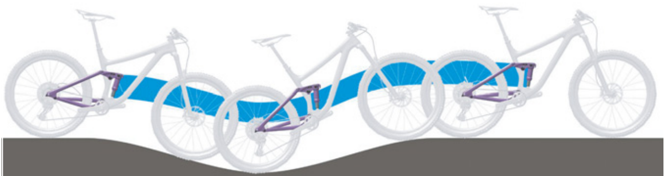
Figure 20: Optimum rear frame damper ride performance on hilly terrain
