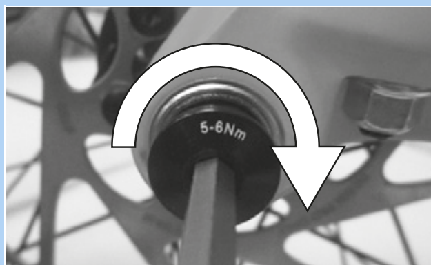
Figure 74: Tightening the securing screw
