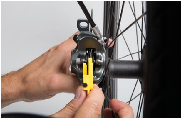
Figure 170: Checking the brake lining when fitted with the help of the transport safety wear gauge
