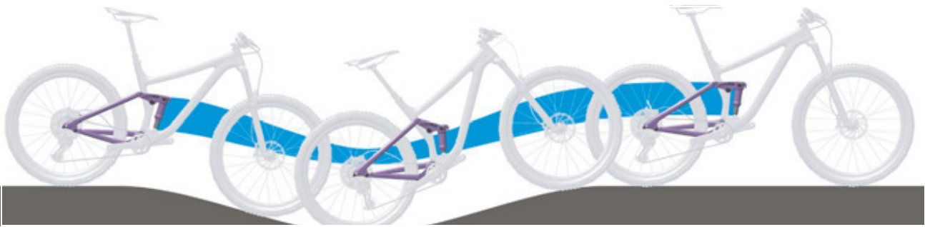
Figure 223: Excessively soft suspension in the rear frame damper on hilly terrain
