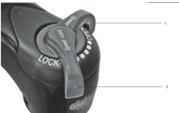
Figure 208: Changing compression adjuster to a harder setting
