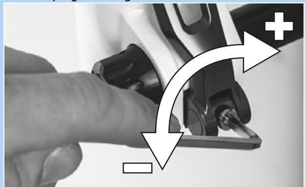
Figure 200: Adjusting the quick release clamping force
