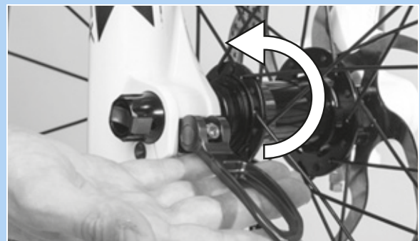
Figure 78: Pressing the quick release lever in the direction of the arrow
