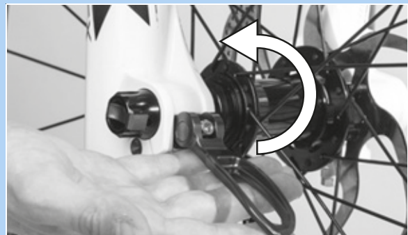
Figure 62: Pressing the quick release lever in the direction of the arrow
