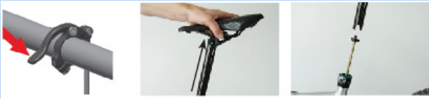
Figure 152: Pulling the seat post out
