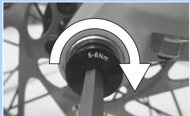
Figure 58: Tightening the securing screw
