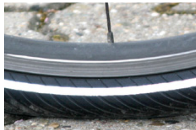
Figure 91: Correct tyre pressure. The tyre is barely deformed under the load of the body weight
