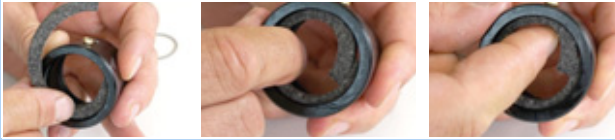
Figure 164: Inserting the felt ring
