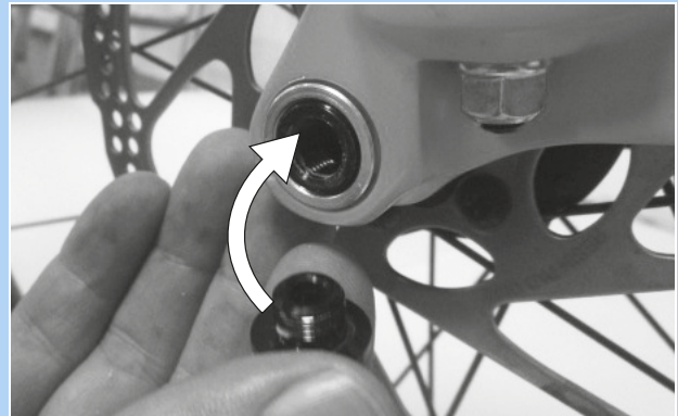
Figure 57: Pushing the quick release lever into the axle
