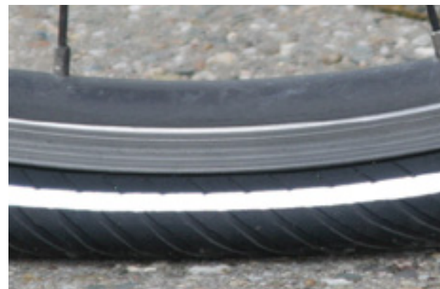
Figure 92: Much too little tyre pressure
