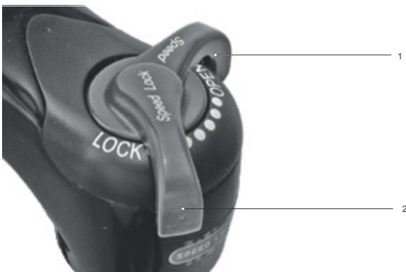
Figure 218: Changing compression adjuster to a harder setting
