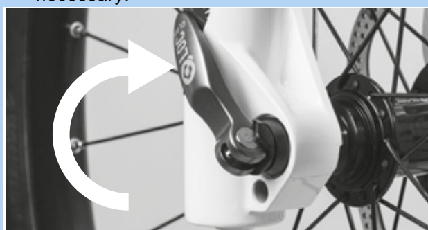
Figure 68: Closing the quick release
