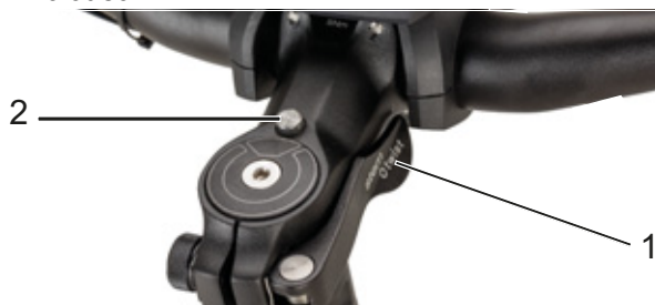
Figure 42: Stem, version II with clamping lever on the stem quick release (1) and unlocking knob (2)
