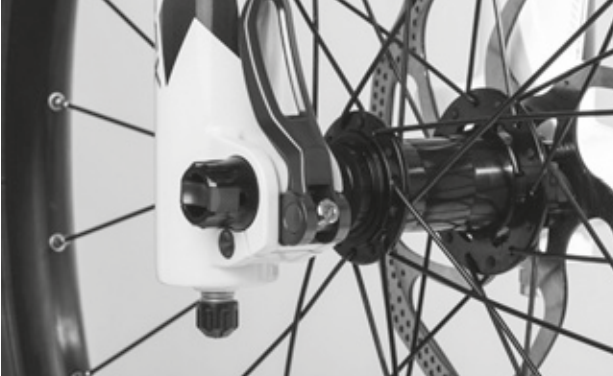
Figure 48: Adjusting the quick release clamping force
