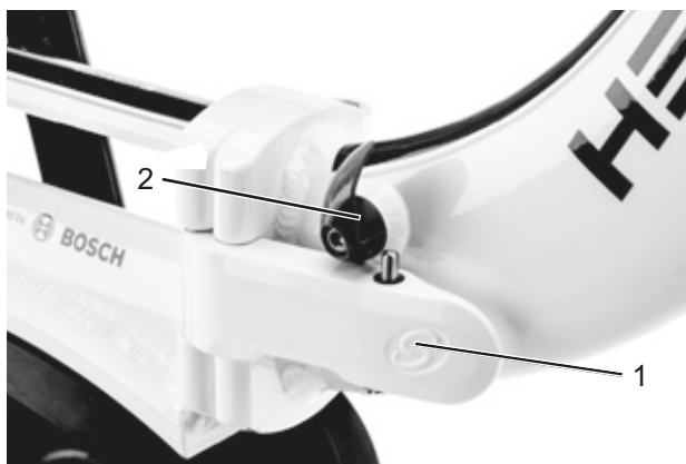
Figure 43: Closed (1) and opened (2) frame locking lever
