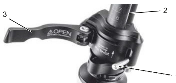
Figure 41: Opened clamping lever on the stem quick release (3) on the stem (2), version I, with locking lever on the stem (1)
