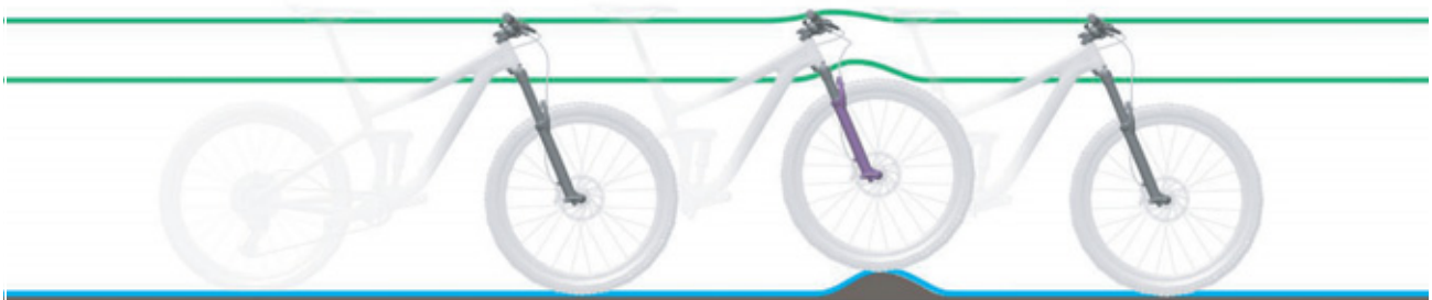
Figure 7: Optimum fork riding performance over bumps
