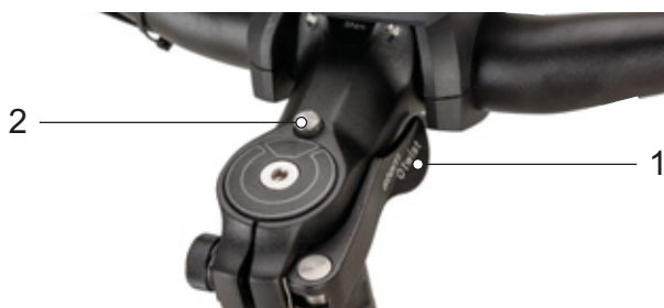
Figure 140: Stem, version II with clamping lever on the stem quick release (1) and unlocking knob (2)
