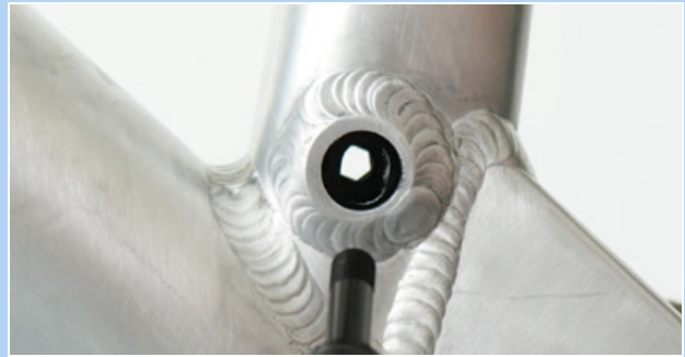
Figure 222: Hole in the Postpin interface
