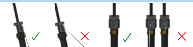
Figure 189: Correct and incorrect Bowden cable
