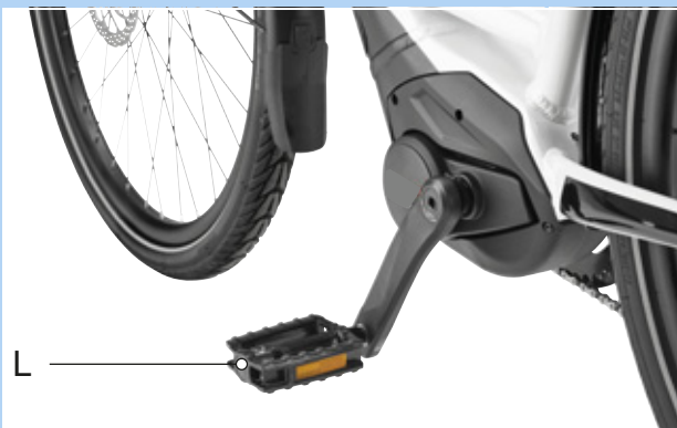
Figure 68: L-pedal in the left-hand crank arm
