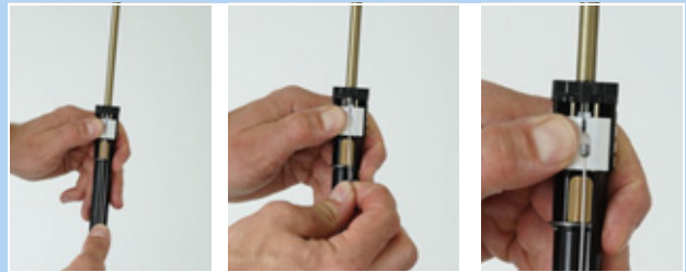
Figure 167: Detaching the Bowden cable
