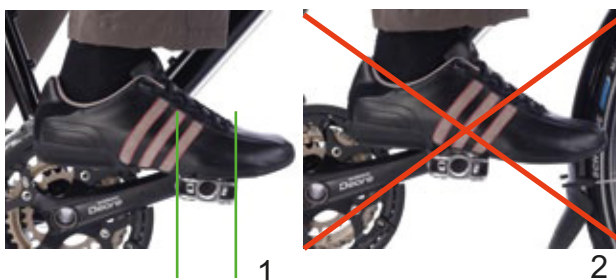
Figure 117: Correct (1) and incorrect (2) foot position on the pedal
