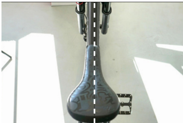
Figure 72: Positioning the saddle in direction of travel
