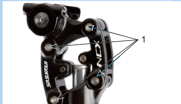
Figure 161: SR Suntour suspension seat post lubrication points
