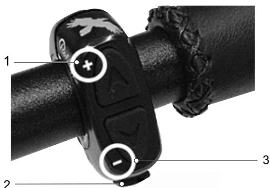
Figure 136: ROHLOFF E-14 handlebar buttons
