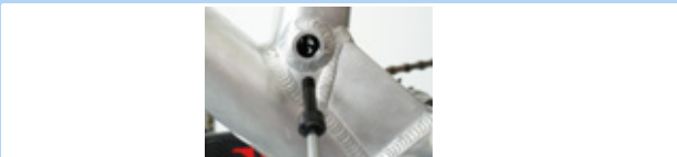
Figure 165: Undoing the Postpin axle
