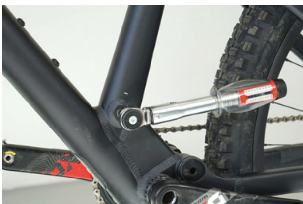
Figure 73: Tightening the seat post axle
