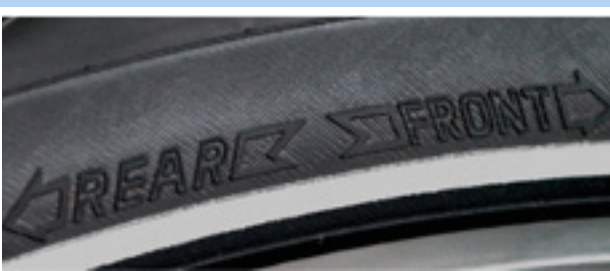
Figure 52: Rotation direction arrow on MTB tyres
