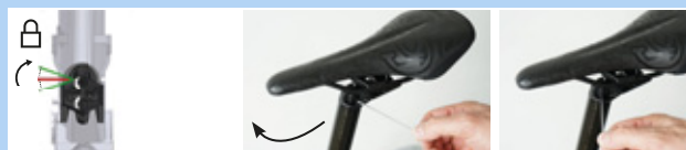
Figure 199: Closing the height adjustment
