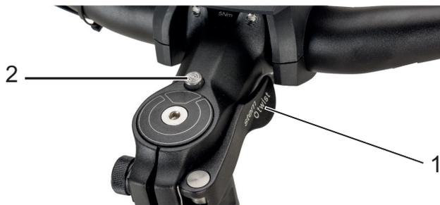
Figure 45: Stem, version II with clamping lever on the stem quick release (1) and unlocking knob (2)
