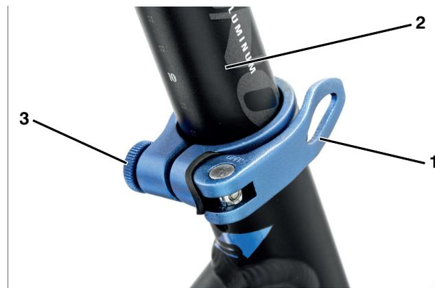
**Figure 21:** Seat post quick release in the final position
