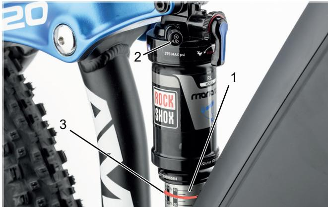
**Figure 28:** Setting the hardness on the suspension damping element
