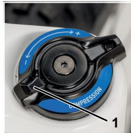
▶ In order to lock the suspension, turn the locking lever in the plus direction.
