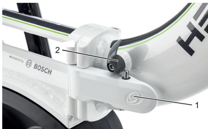
**Figure 46:** Frame, with closed frame clamping lever (1) and open frame locking lever (2)
