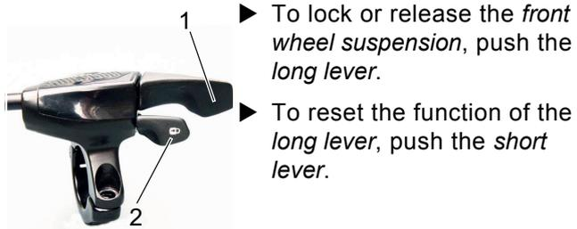
Figure 38: Fork lock on handlebars, version III, with long lever (1) and short lever (2), example
