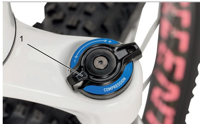
**Figure 31:** Compression damper with locking lever (1), example
