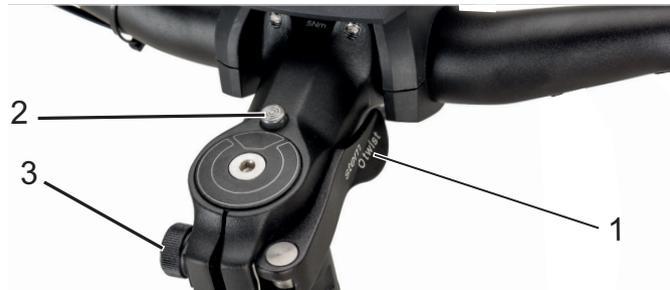
Figure 24: Stem, version II with clamping lever (1), unlocking knob (2) and knurled nut (3)
