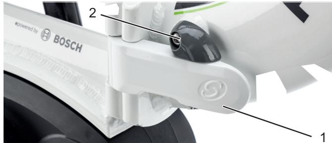
**Figure 47:** Frame, with closed frame clamping lever (1) and closed frame locking lever (2)
