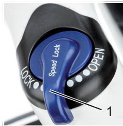
► In order to lock the *front wheel suspension*, shift the LOCKING LEVER to the LOCK position.
