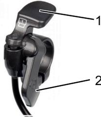
▶ To release the *front wheel suspension*, push the side unlocking lever.
