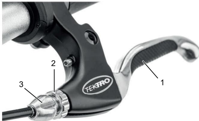
Figure 66: Brake lever (1), lock nut (2) and setting bolt (3) of the cable-operated rim brake
