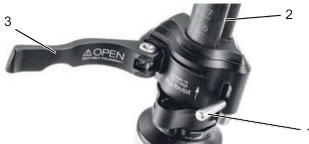
**Figure 44:** Opened clamping lever on the stem quick release (3) on the stem (2), version I, with locking lever on the stem (1)
