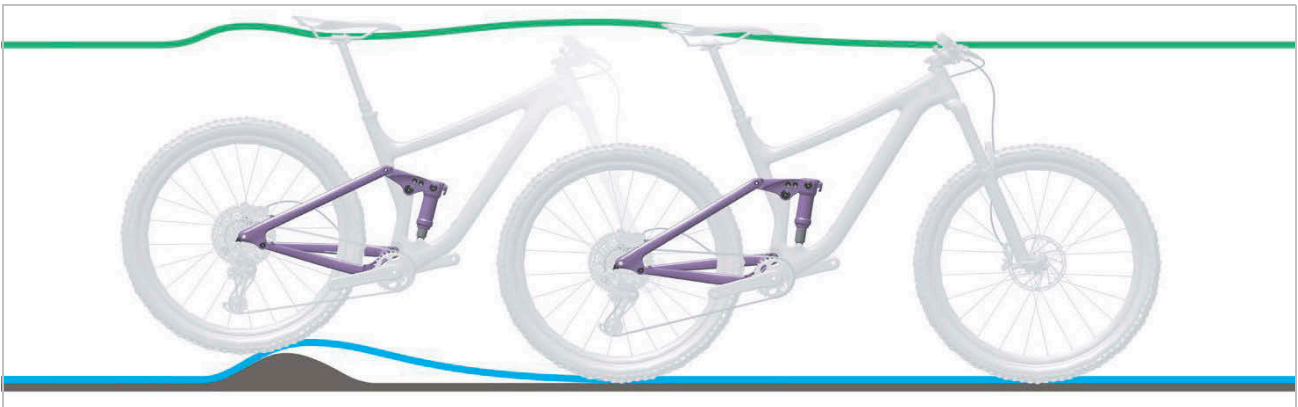
Figure 282: Excessively hard damping in the rear frame damper on bumps
