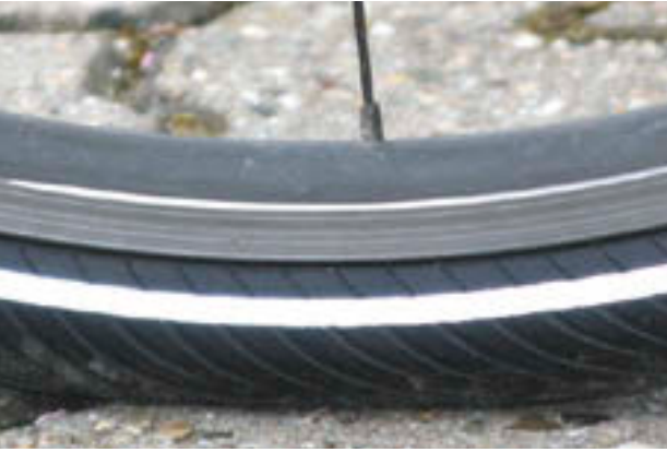
Figure 129: Correct tyre pressure. The tyre is barely deformed under the load of the body weight
