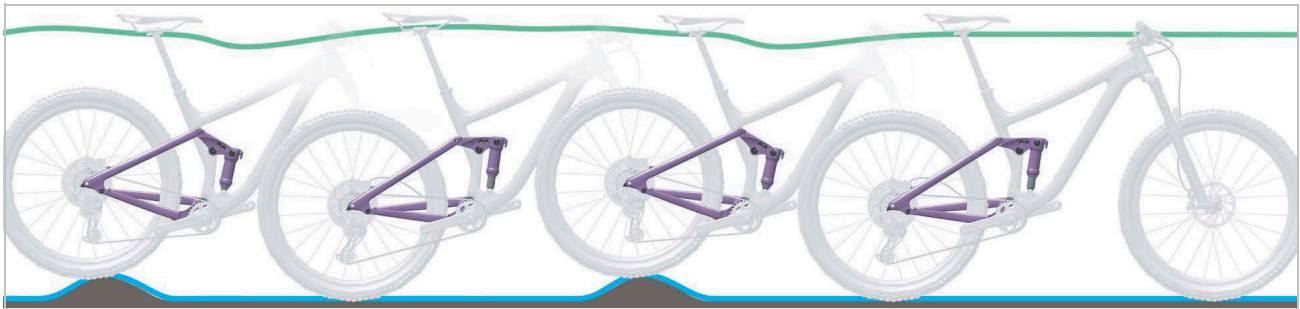
Figure 6: Optimum rear frame damper ride performance
