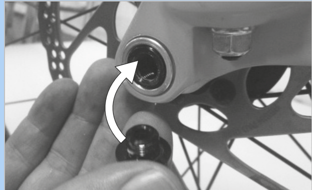
Figure 91: Inserting the securing screw
