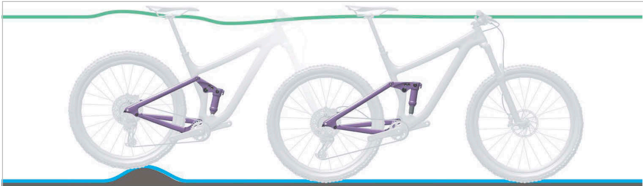
Figure 193: Optimum rear frame damper ride performance over bumps
