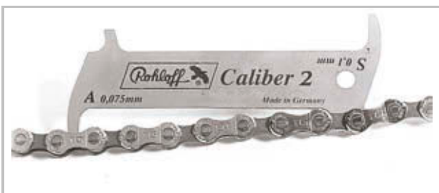
Figure 230: Example of a ROHLOFF gauge
