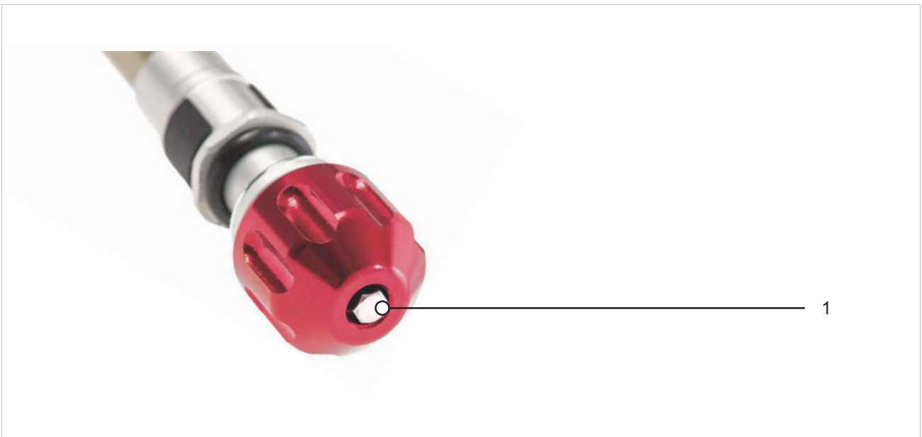
Figure 265: Example of SR SUNTOUR rebound adjuster (fork) (1)
