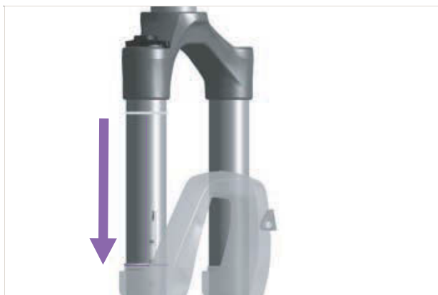
Figure 145: Moving the O-ring on the suspension fork
