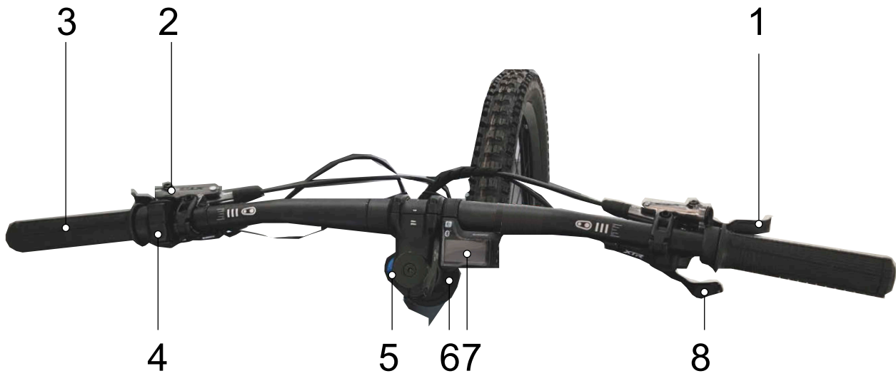
Figure 72: Detailed view of handlebars with SHIMANO SC-E800 on-board computer, used as example
