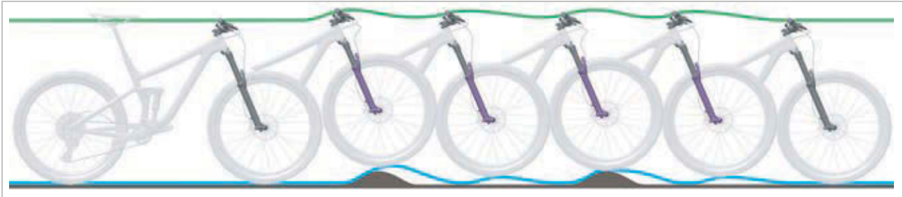
Figure 262: Suspension fork rebounding too quickly
