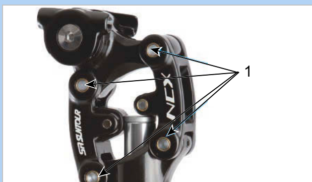
Figure 255: SR SUNTOUR suspension seat post lubrication points
