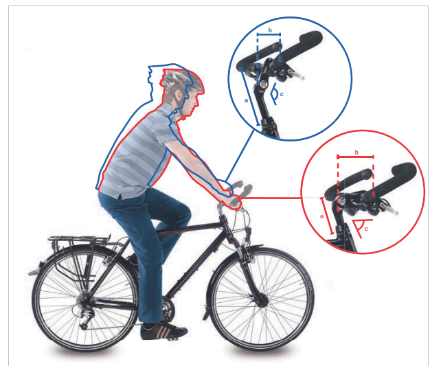
Figure 127: City bike (blue) and trekking bike position (red) by changing the angle
