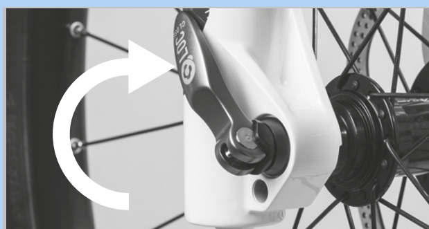
Figure 102: Closing the quick release
