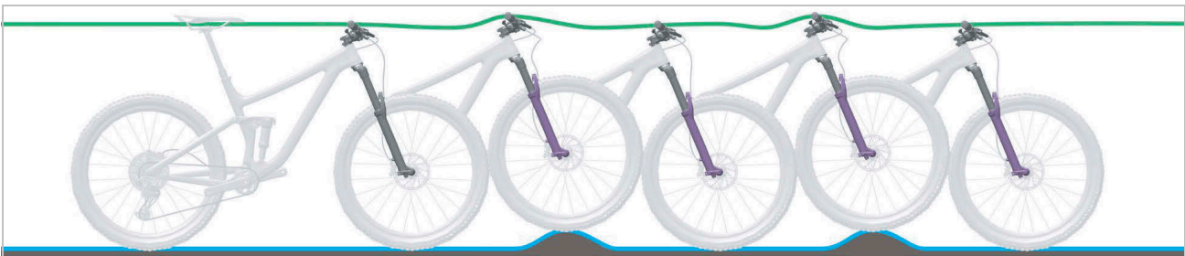
Figure 21: Optimum suspension fork ride performance
