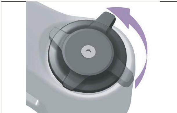
Figure 275: Adjust the compression adjuster so that it is softer
