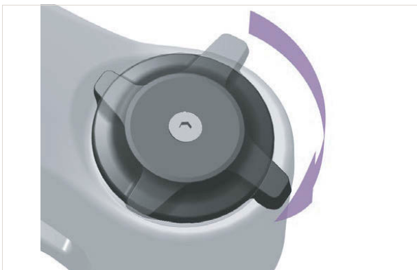
Figure 273: Adjust the compression adjuster so that it is harder
