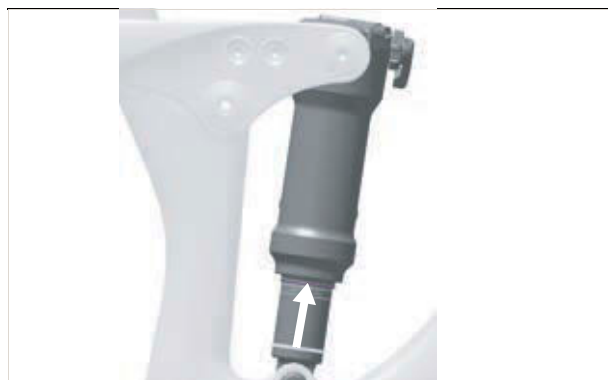
Figure 151: Moving the O-ring on the rear frame damper
