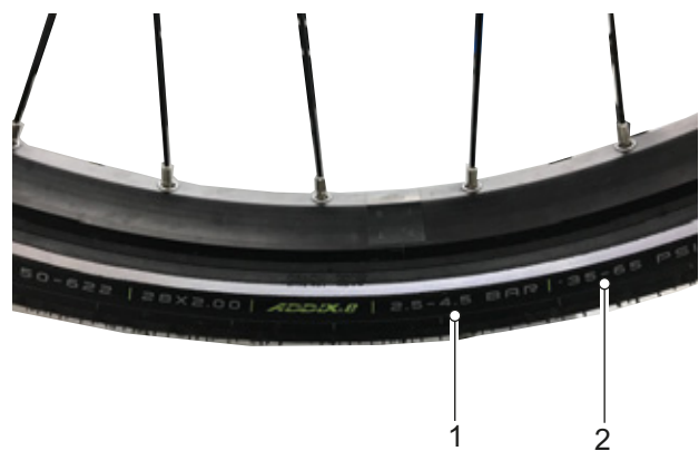
Figure 155: Tyre pressure in bar (1) and psi (2)
