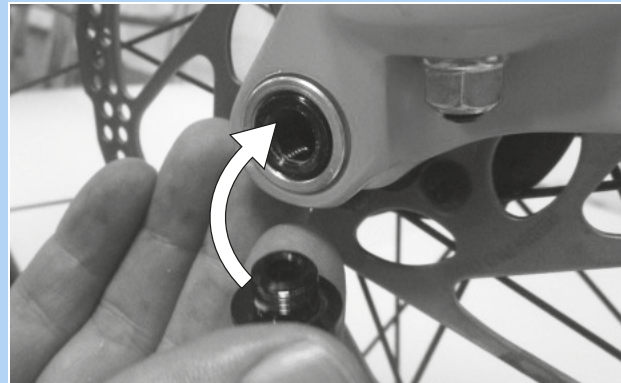
Figure 68: Pushing the quick release lever into the axle
