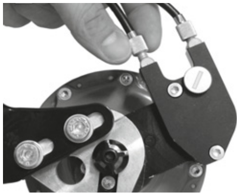
Figure 162: The tension adjuster on Rohloff hub versions with external switch control is located on the cable box positioned on the left-hand side
