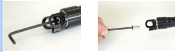
Figure 185: Unscrewing the valve cap
