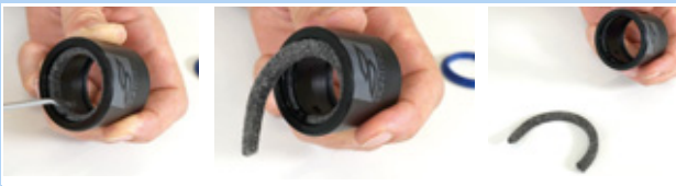
Figure 215: Removing the felt ring
