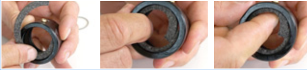
Figure 182: Inserting the felt ring
