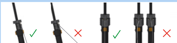
Figure 196: Correct and incorrect Bowden cable
