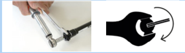
Figure 191: Setting in a clockwise direction
