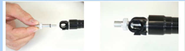
Figure 186: Screwing the valve adapter in
