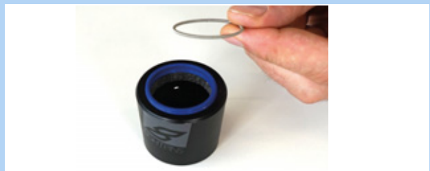
Figure 213: Removed spring washer
