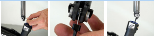
Figure 227: Attaching and pushing in the seat post
