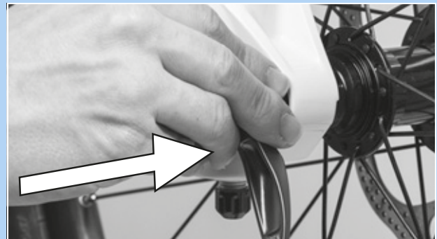
Figure 77: Inserting the quick release in the direction of the arrow
