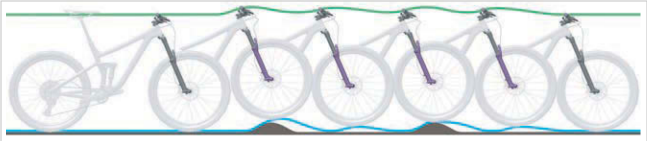
Figure 188: Suspension fork rebounding too quickly
