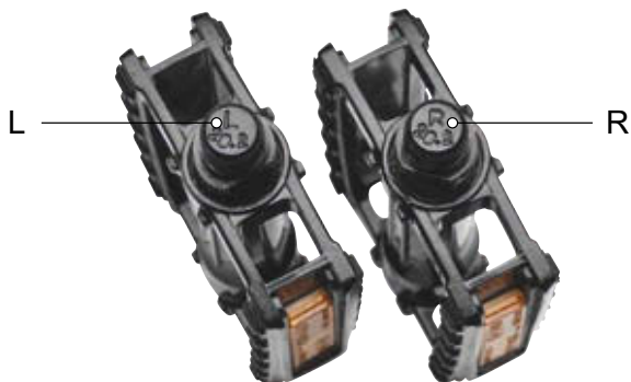
Figure 83: Example of markings on pedals
