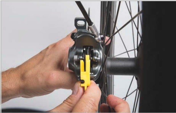
Figure 155: Checking the brake lining when fitted with the help of the transport safety wear gauge
