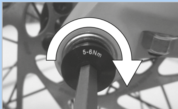
Figure 70: Tightening the securing screw
