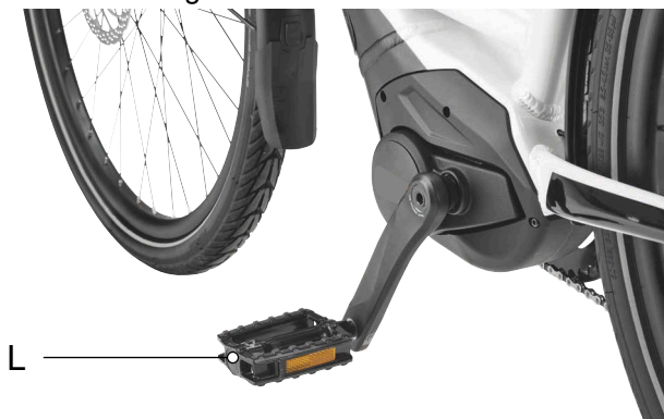
Figure 84: L pedal in the left-hand crank arm
