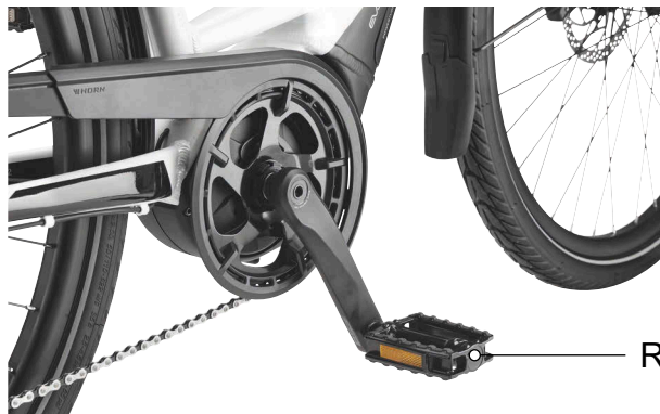
Figure 85: R pedal in the right-hand crank arm
