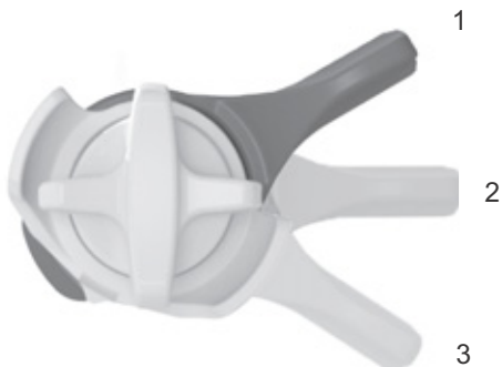
Figure 85: FOX compression adjuster on the rear frame damper with the OPEN (1), MEDIUM (2) and HARD (3) positions
