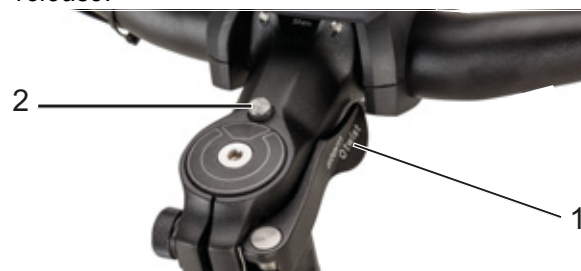
Figure 72: Stem, version II with clamping lever on the stem quick release (1) and unlocking knob (2)
