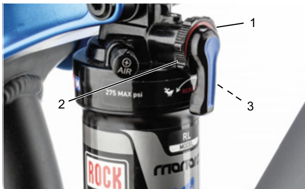
Figure 78: Setting the rebound damper strength on the rear frame damper setting wheel (1)
