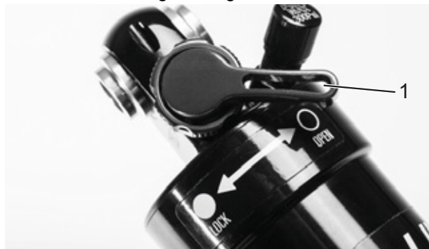
Figure 76: Suntour compression adjuster open (1)
