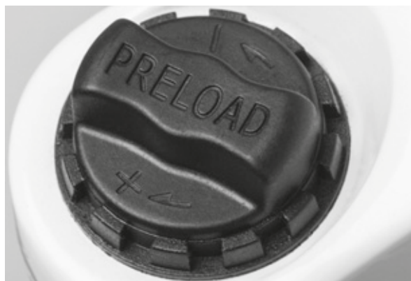
Figure 56: Negative deflection setting wheel on the suspension fork crown
