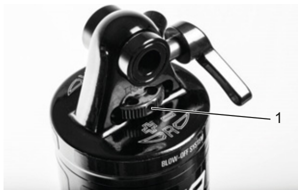
Figure 60: Suntour rebound adjuster wheel (1) on the rear frame damper
