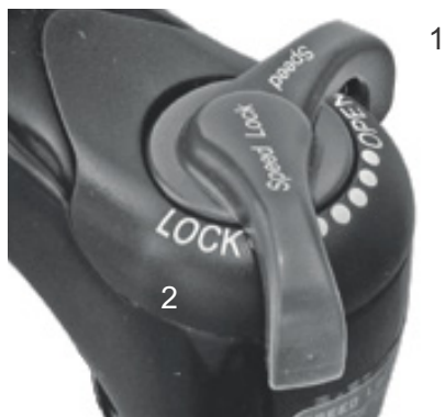
Figure 75: Suntour compression adjuster with the OPEN (1) and LOCK (2) positions
