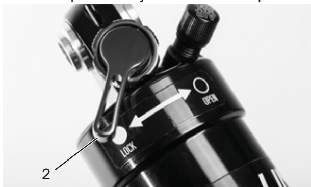
Figure 77: Suntour compression adjuster closed (2)
