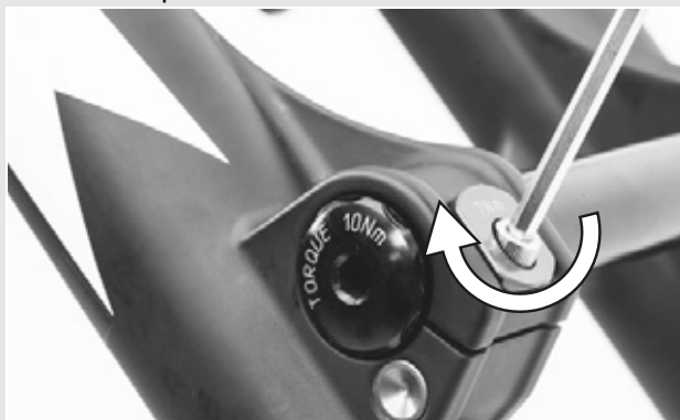
Figure 31: Tightening the axle
