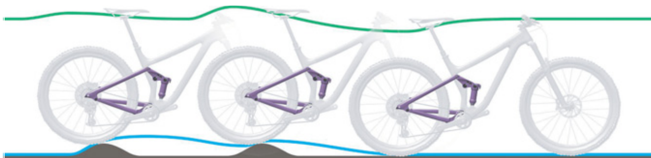
Figure 265: Rear frame damper rebounding too slowly
