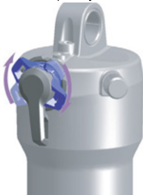
Figure 121: Changing compression adjuster to a harder setting
