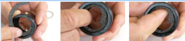
Figure 225: Inserting the felt ring
