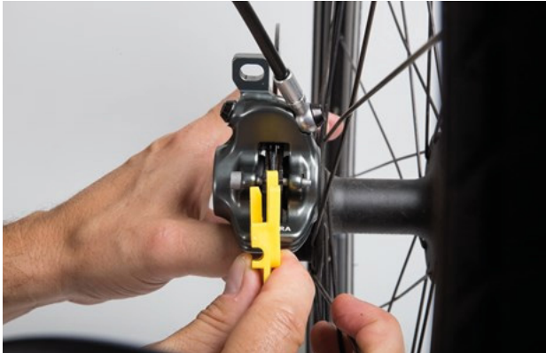
Figure 166: Checking the brake lining when fitted with the help of the transport safety wear gauge
