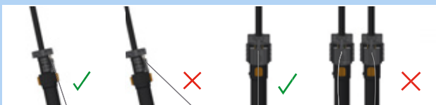
Figure 204: Correct and incorrect Bowden cable
