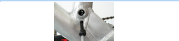
Figure 180: Undoing the Postpin axle
