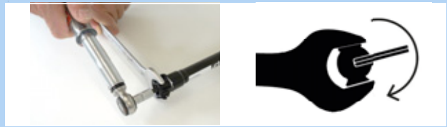
Figure 199: Setting in a clockwise direction
