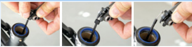
Figure 218: Removing the Bowden cable
