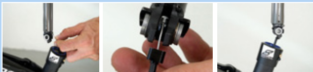
Figure 235: Attaching and pushing in the seat post
