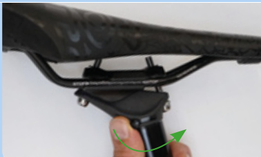
Figure 228: Opening the height adjustment
