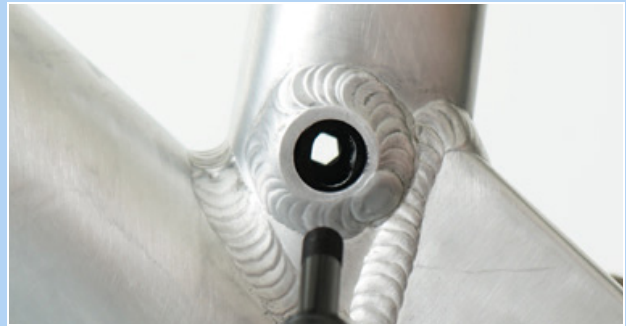
Figure 237: Hole in the Postpin interface
