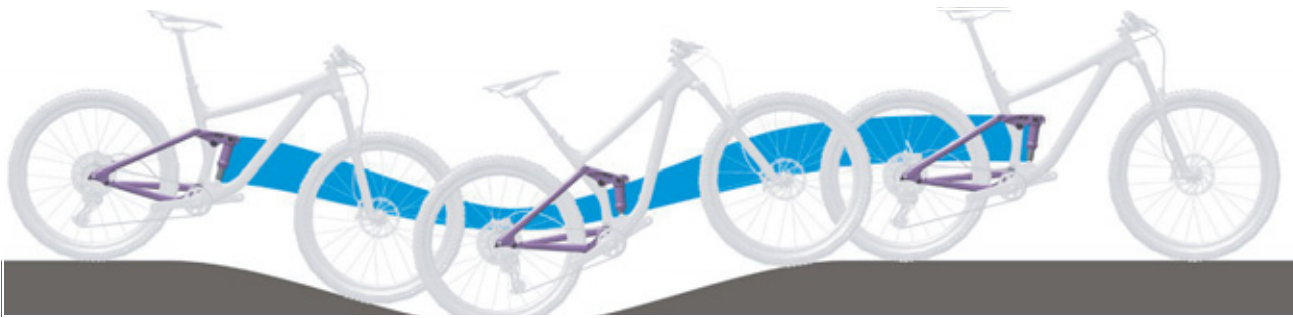
Figure 267: Excessively soft suspension in the rear frame damper on hilly terrain
