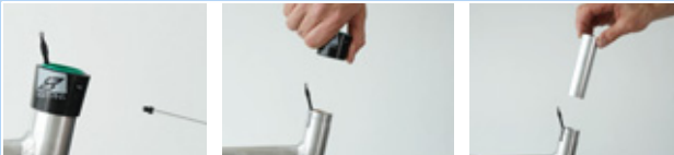
Figure 185: Removing the outer sleeve and slide bushing
