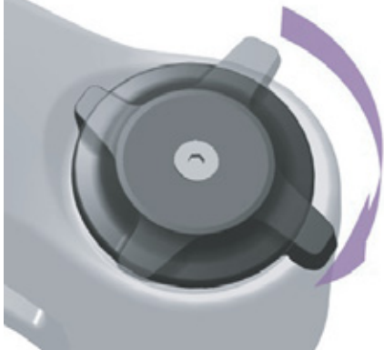
Figure 150: Changing compression adjuster to a harder setting
