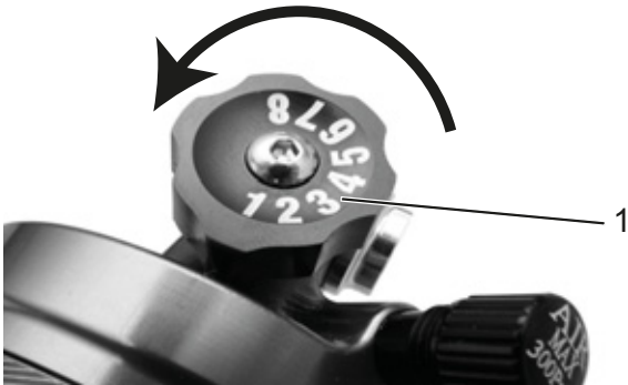
Figure 118: Suntour compression adjuster (1) on the rear frame damper
