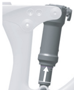
Figure 113: Moving the O-ring on the rear frame damper
