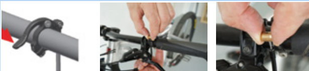
Figure 179: Removing the cartridge
