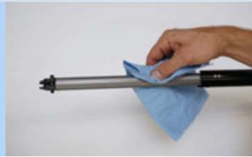
Figure 230: Cleaning the longitudinal groove
