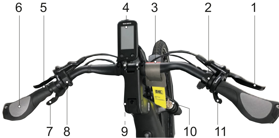
Figure 38: Detailed view of handlebars with SHIMANO SC-E5003 on-board computer, used as example
