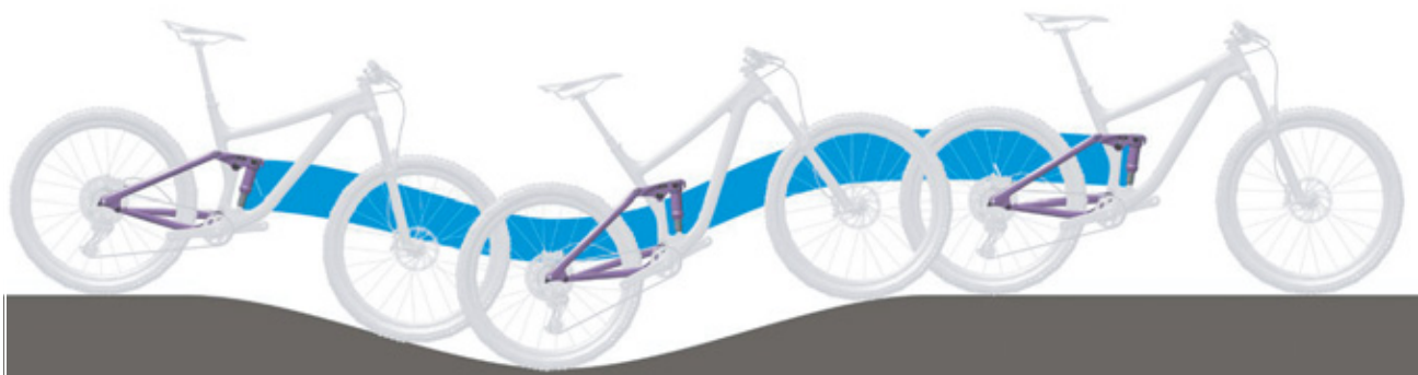
Figure 19: Optimum rear frame damper ride performance on hilly terrain
