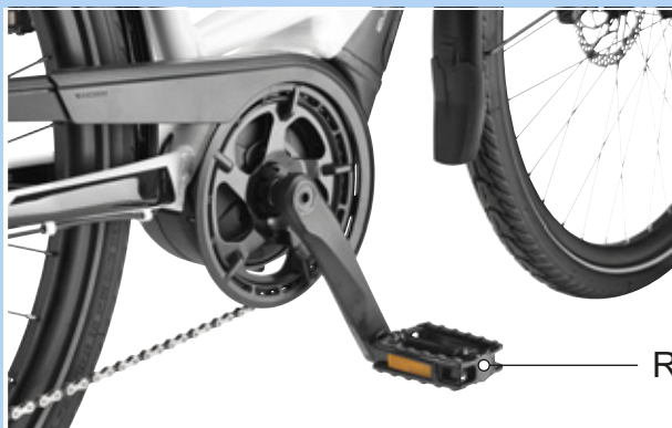
Figure 67: R-pedal in the right-hand crank arm
