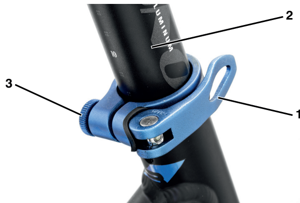
Figure 17: Seat post quick release in the final position
