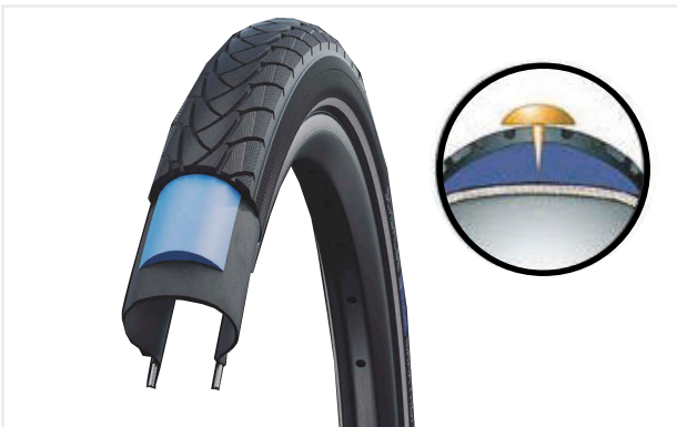
Figure 13: Effect of puncture protection belt
