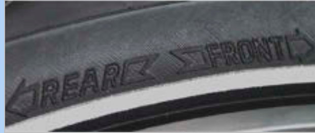
Figure 41: Rotation direction arrow on MTB tyres
