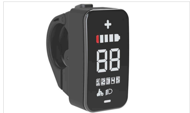
Figure 31: On-board computer DP E160.CAN
