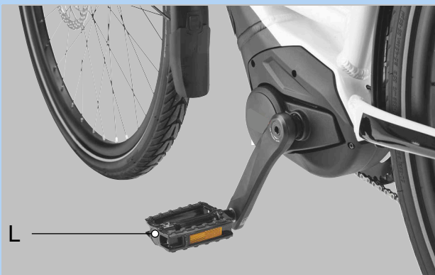
Figure 43: L-pedal in the left-hand crank arm
