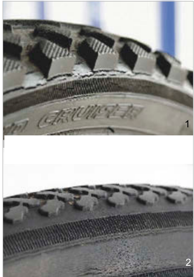
Figure 103: Examples of fatigue cracks (1) and ageing cracks (2)
