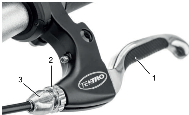
Figure 36: Brake lever (1), lock nut (2) and setting bolt (3) of the cable-operated rim brake
