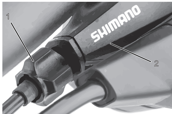
Figure 34: Adjusting sleeve (1) for the single-cable cable-operated gear shift with gear shift housing (2), example
