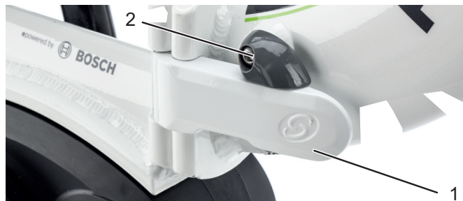
Figure 26: Frame, with closed frame clamping lever (1) and closed frame locking lever (2)
