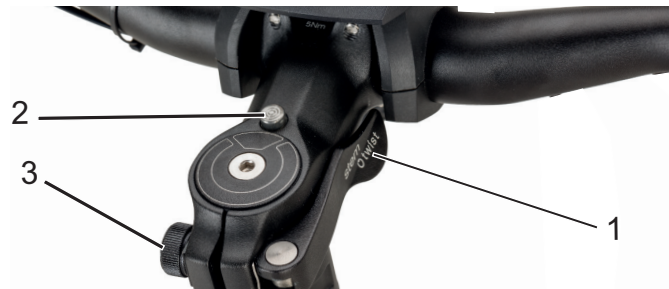
Figure 18: Stem, version II with clamping lever (1), unlocking knob (2) and knurled nut (3)
