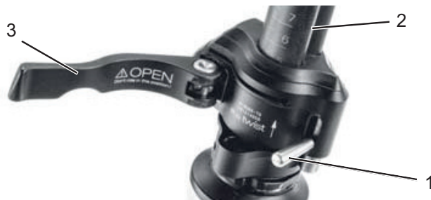
Figure 23: Opened clamping lever on the stem quick release (3) on the stem (2), version I, with locking lever on the stem (1)
