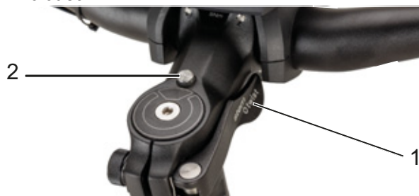
Figure 58: Stem, version II with clamping lever on the stem quick release (1) and unlocking knob (2)
