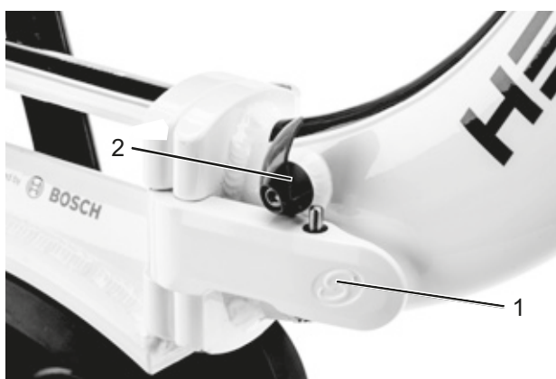
Figure 59: Closed (1) and opened (2) frame locking lever
