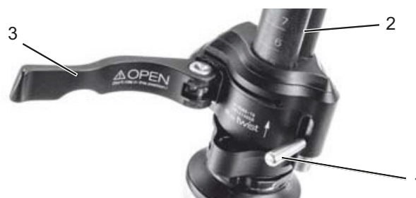
Figure 57: Opened clamping lever on the stem quick release (3) on the stem (2), version I, with locking lever on the stem (1)
