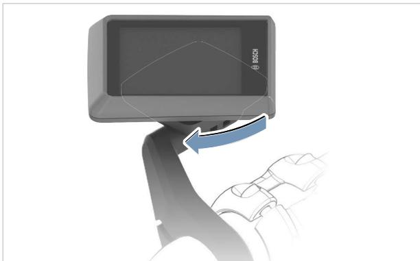
Figure 135: Turning the display clockwise
