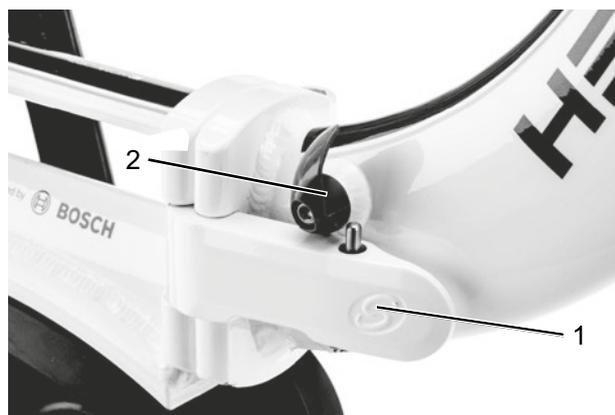
Figure 171: Closed (1) and opened (2) frame locking lever
