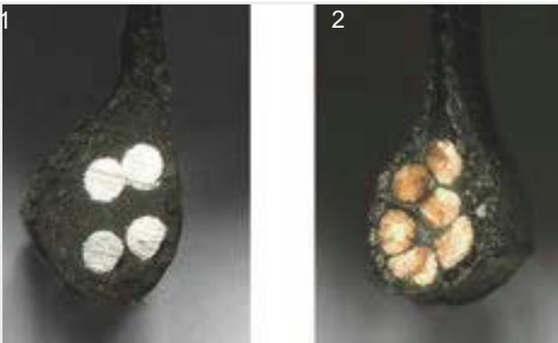
Figure 27: Steel bead core (1) and Kevlar bead core (2)
