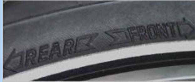
Figure 68: Rotation direction arrow on MTB tyres
