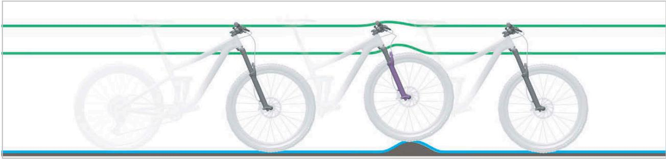
Figure 17: Optimum suspension fork ride performance over bumps
