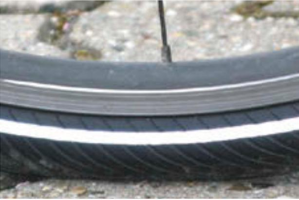
**Figure 109: Correct tyre pressure. The tyre is barely deformed under the load of the body weight**
