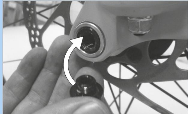
Figure 71: Inserting the securing screw
