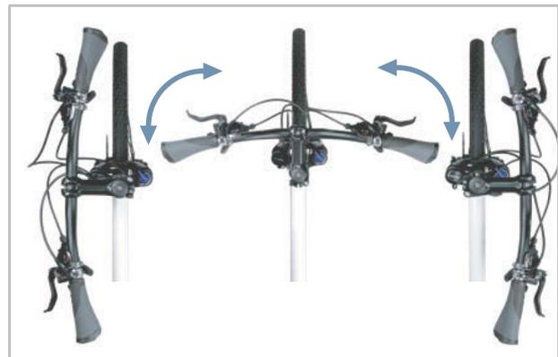
Figure 9: Twist function, using BY.SCHULZ as an example
