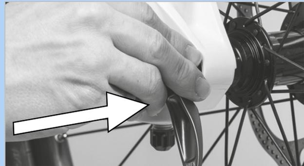
Figure 80: Inserting the quick release in the direction of the arrow
