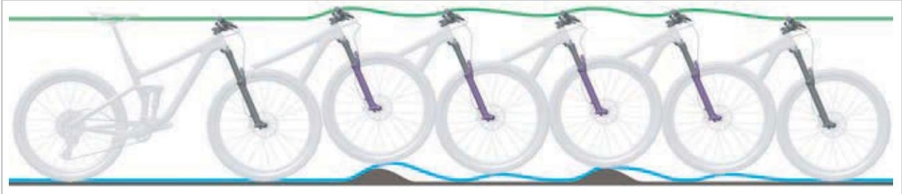
Figure 205: Suspension fork rebounding too quickly
