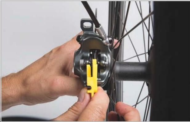
Figure 182: Checking the brake lining when fitted with the help of the transport safety wear gauge
