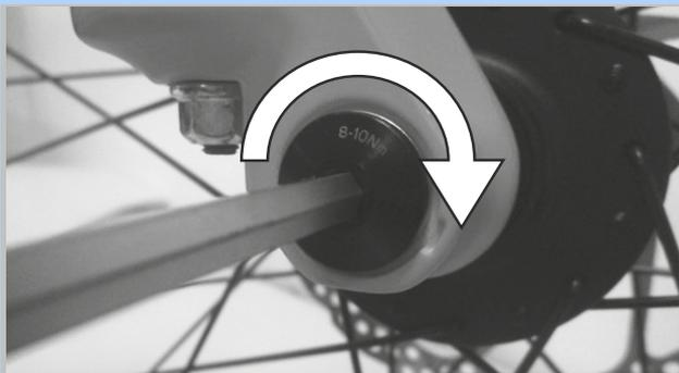
Figure 70: Tighten the axle in the direction of the arrow
