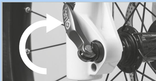
Figure 82: Closing the quick release
