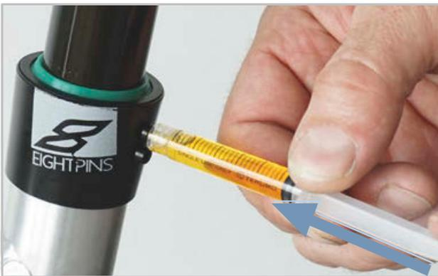
Figure 178: Lubricating the Eightpins seat post
