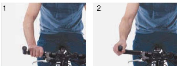
Figure 153: Grip positions on a bar end
