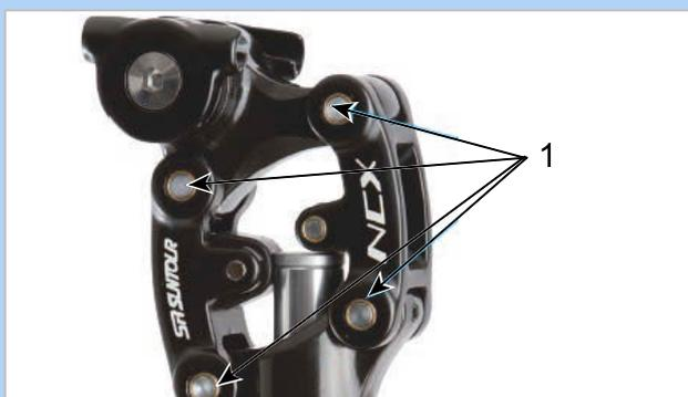
Figure 202: SR SUNTOUR suspension seat post lubrication points
