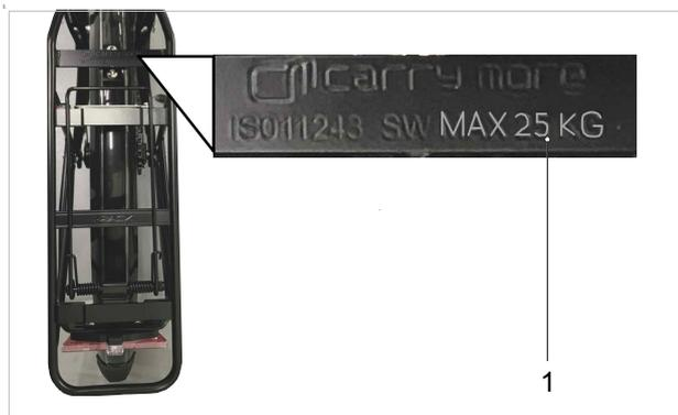
Figure 149: The maximum load bearing capacity is indicated on the pannier rack
