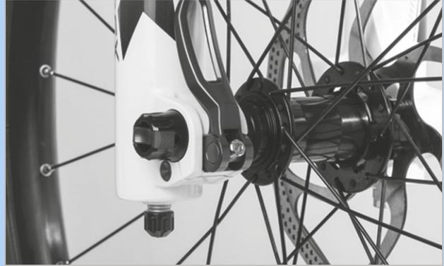
Figure 200: Adjusting the quick release clamping force
