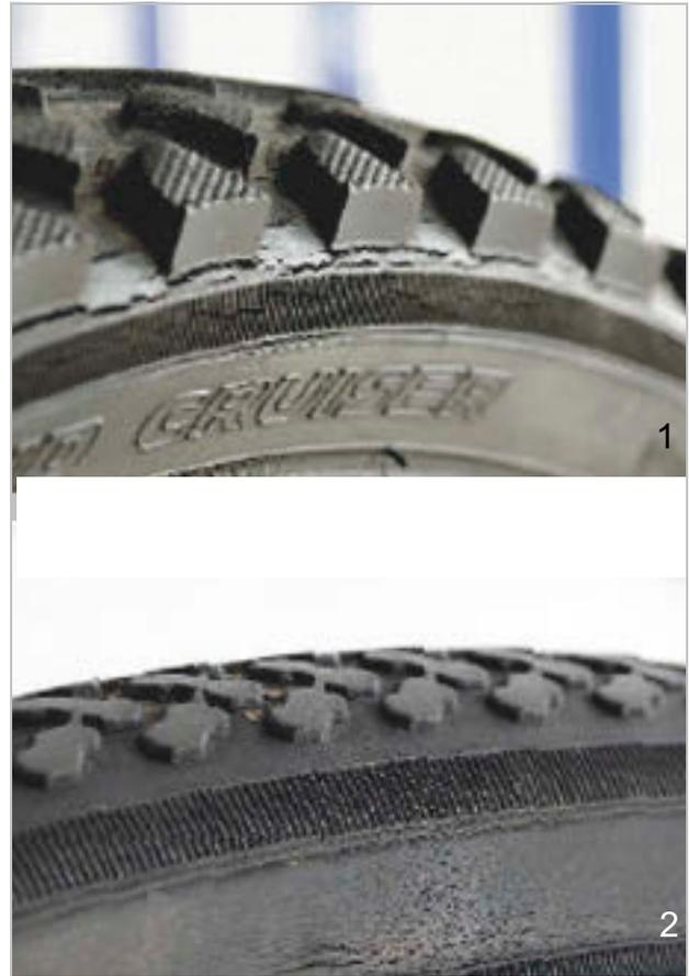
Figure 181: Examples of fatigue cracks (1) and ageing cracks (2)
