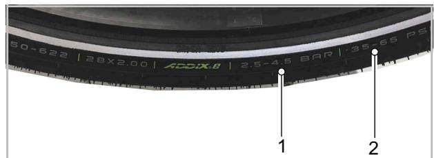
Figure 179: Tyre pressure specification in bar (1) and psi (2)
