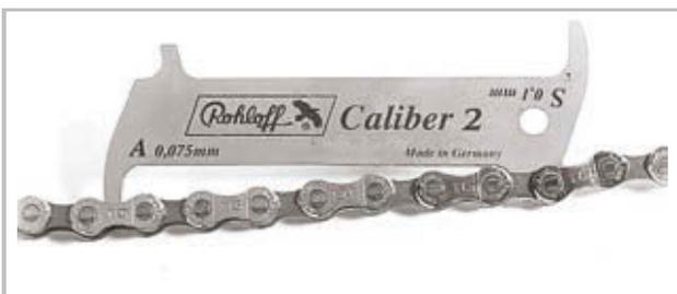
Figure 188: Example of a ROHLOFF gauge
