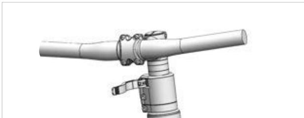
Figure 146: Example of All Up with open stem clamping lever
