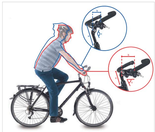
Figure 107: City bike (blue) and trekking bike position (red) by changing the angle
