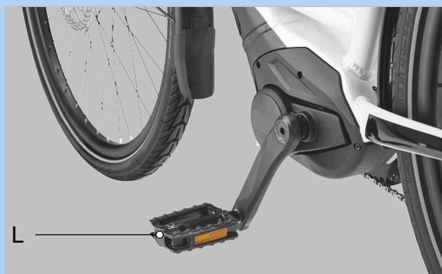
Figure 84: L-pedal in the left-hand crank arm
