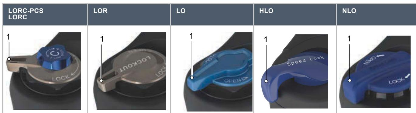
Table 47: Lockout on the crown on SR Suntour suspension forks
