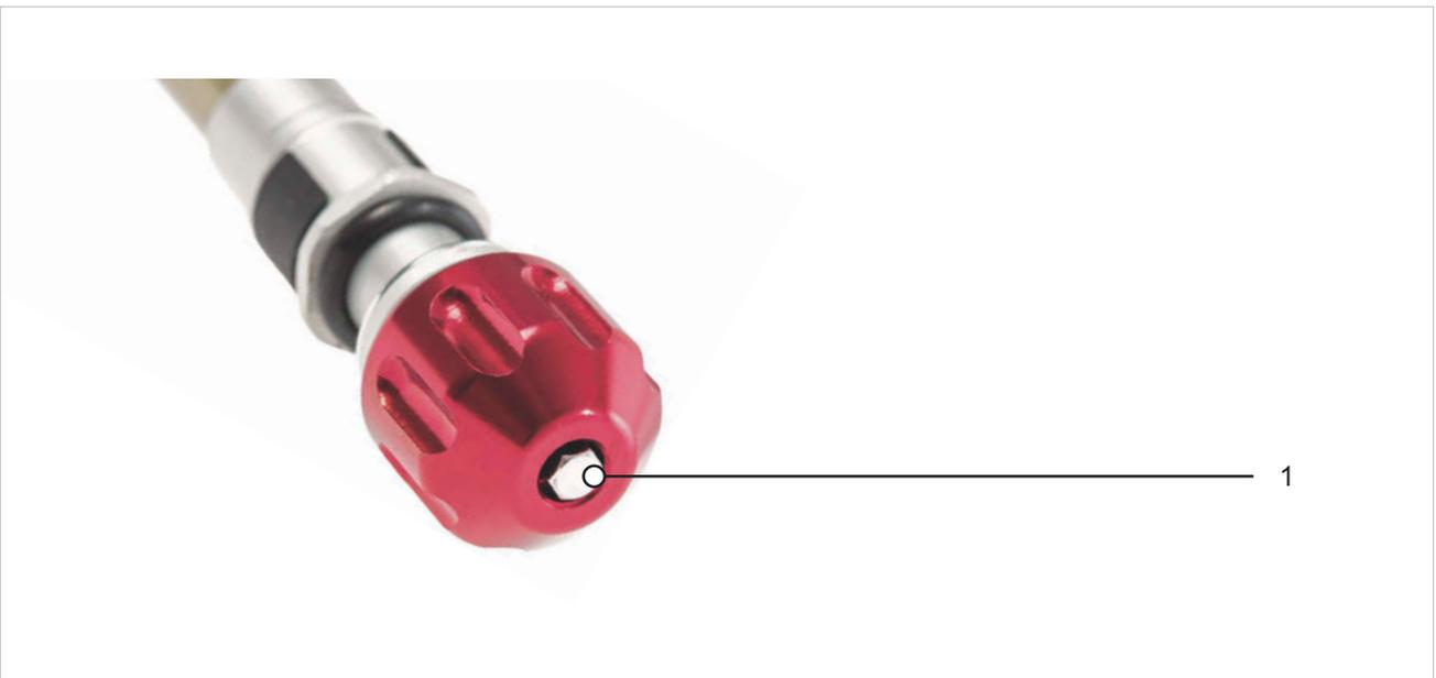
Figure 208: Example of SR SUNTOUR rebound adjuster (fork) (1)
