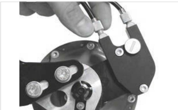
Figure 197: The tension adjuster on ROHLOFF hub versions with external switch control is located on the cable box positioned on the left-hand side
