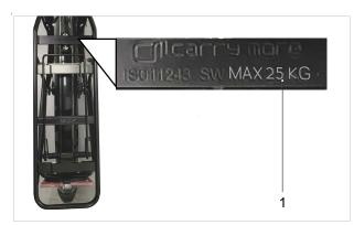
Figure 149: The maximum load bearing capacity is indicated on the pannier rack
