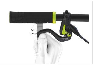
Figure 114: Handbrake positioning
