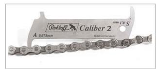
Figure 188: Example of a ROHLOFF gauge
