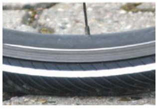
Figure 109: Correct tyre pressure. The tyre is barely deformed under the load of the body weight
