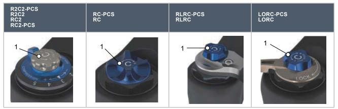
Table 50: Low-speed lever (1) on the fork crown on the SR Suntour suspension fork
