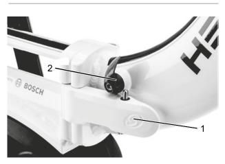
Figure 171: Closed (1) and opened (2) frame locking lever
