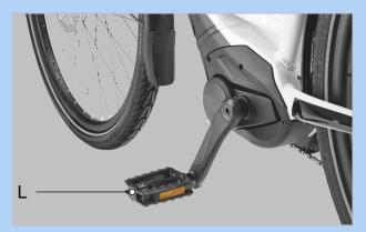
Figure 84: L-pedal in the left-hand crank arm
