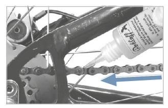
Figure 177: Lubricating the chain
