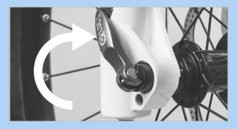
Figure 82: Closing the quick release
