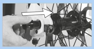
Figure 73: Inserting the cross axle in the direction of the arrow
