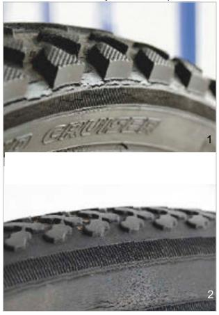
Figure 181: Examples of fatigue cracks (1) and ageing cracks (2)  $% \left( 2\right) =0$
