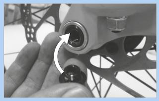
Figure 71: Inserting the securing screw
