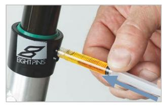
Figure 178: Lubricating the Eightpins seat post
