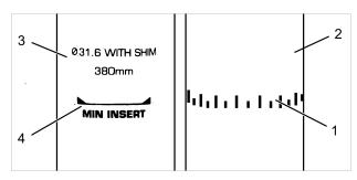
Figure 97: Detailed view of the seat post – examples of the minimum insertion depth marking
