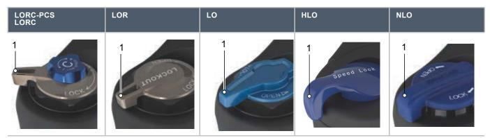
Table 51: Lockout on the fork crown on SR Suntour suspension forks
