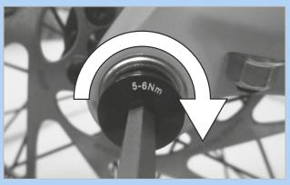
Figure 72: Tightening the securing screw
