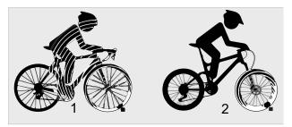
Figure 11: Without suspension (1) and with suspension (2)
