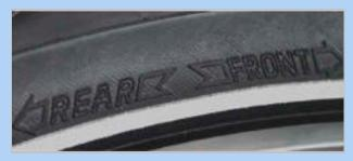
Figure 68: Rotation direction arrow on MTB tyres
