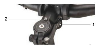
Figure 170: Stem, version II with clamping lever on the stem quick release (1) and unlocking knob (2)
