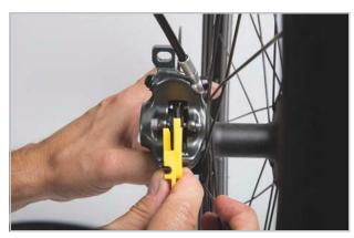
Figure 182: Checking the brake lining when fitted with the help of the transport safety wear gauge
