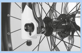
Figure 200: Adjusting the quick release clamping force
