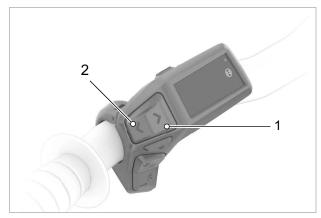
Figure 156: Position of increase brightness button (2) and decrease brightness button (1)
