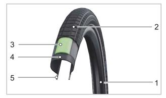
Figure 26: Structure of tube-type tyre
