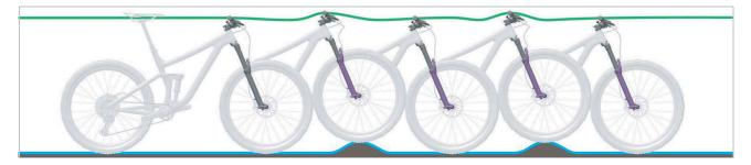
Figure 18: Optimum suspension fork ride performance
