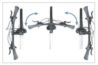
Figure 9: Twist function, using BY.SCHULZ as an example
