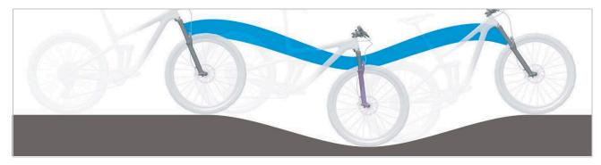
Figure 16: Optimum suspension fork ride performance on hilly terrain
