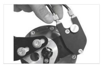
Figure 197: The tension adjuster on ROHLOFF hub versions with external switch control is located on the cable box positioned on the left-hand side
