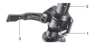
Figure 169: Opened clamping lever on the stem quick release (3) on the stem (2), version I, with locking lever on the stem (1)
