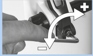
Figure 201: Adjusting the quick release clamping force
