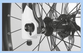
Figure 77: Perfect position for the clamping lever
