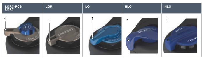
Table 47: Lockout on the crown on SR Suntour suspension forks
