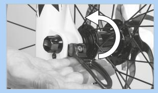
Figure 76: Pressing the quick release lever in the direction of the arrow
