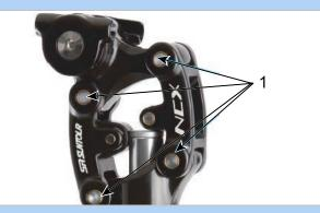
Figure 202: SR SUNTOUR suspension seat post lubrication points
