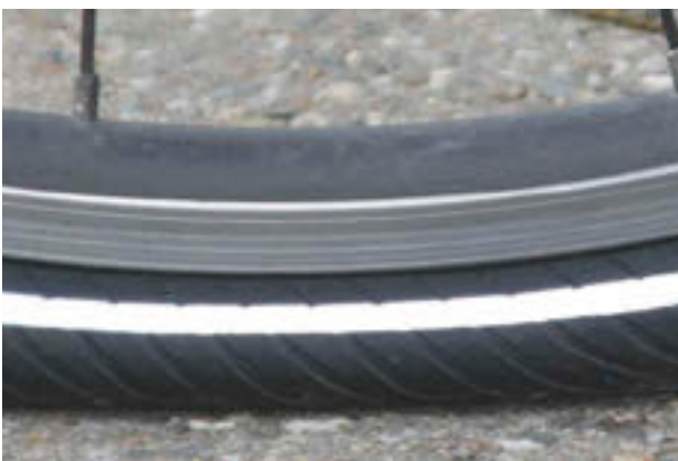
Illustration 139 : Pression largement insuffisante
